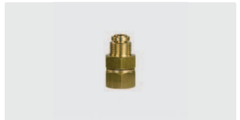
3/8" AG : 1/4" IG. Messing. Max. 220 bar / 90 °C
