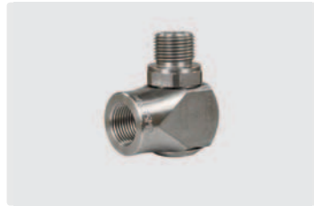
3/8" IG : 3/8" AG. DN 6. Max. 400 bar / 30 U/min / 90 °C
